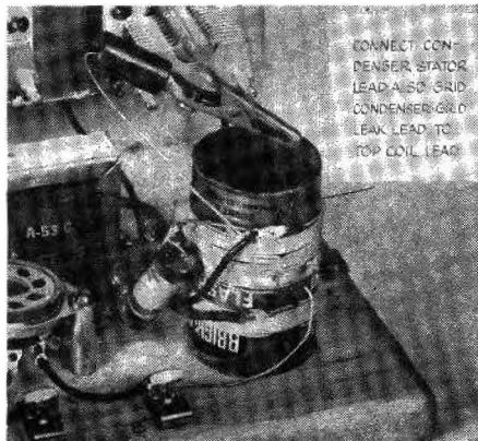
10. Fasten the coil to the base piece with model airplane cement. Solder the leads as indicated in the previous photo. Note directions carefully.
